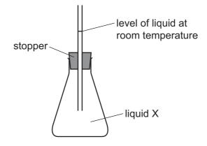
When the flask is placed in warm water, the liquid rises higher up the tube. When the flask is put in cold water, the liquid drops below the original level in the tube.
